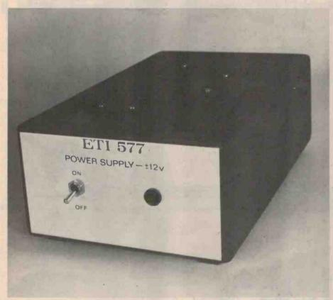
Our prototype was housed in a diecast box to match that used for our Series 4000 moving-coil cartridge preamp, although any suitable box may be used if the power supply is intended for another application. Scotchcal front panels should be available from kit suppliers or separately from Radio Despatch Service in Sydney.
