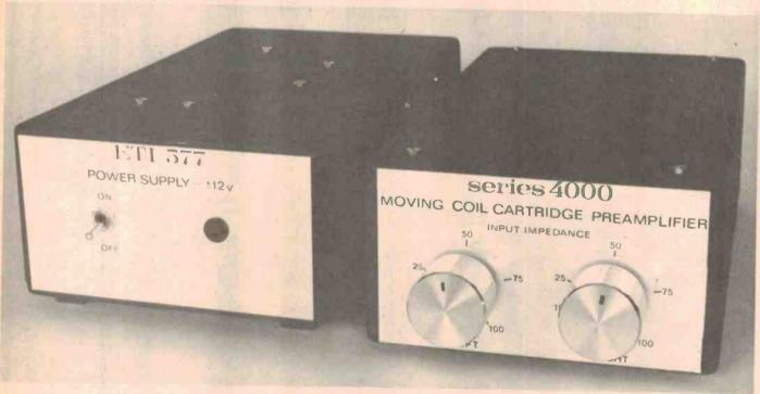
OVER THE LAST several years there has been a dramatic increase in the number of moving coil cartridges released. The design of this type of cartridge results in a number of advantages over the more usual phono cartridge which works on a moving magnet principle.
