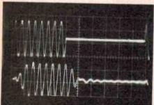
Tone-burst response at 40 Hz (for 90 dB SPL at two metres).
