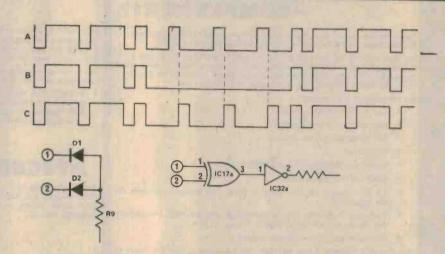
exclusive OR gate, followed by an inverter. As both the ex-OR and the inverter are available spare in packages on the VDU board, this modification can be made without extra parts or cost!
