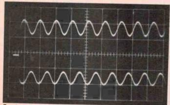
Transient overload recovery test. Upper trace, input - lower trace, output. (1 ms/div.).
