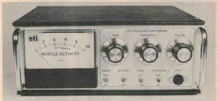
OUR PROTOTYPE was housed in a Horwood instrument case measuring 254 mm wide by 203 mm deep by 102 mm high. These are available from quite a few component suppliers but any box with similar dimensions should suffice. The advantage of this particular case is that it is supplied with steel top, bottom and side panels which provide better shielding from stray hum fields than does aluminium.
