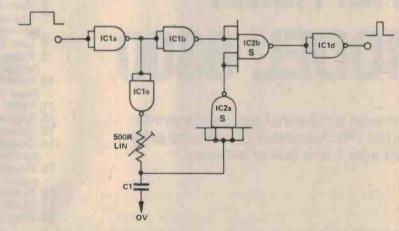
When the input pulse is applied, the output of IC1c starts to rise, but the output of the circuit remains low because of the high on the output of IC2a. When C1 charges to the threshold voltage of IC2a, the output of IC2a will
