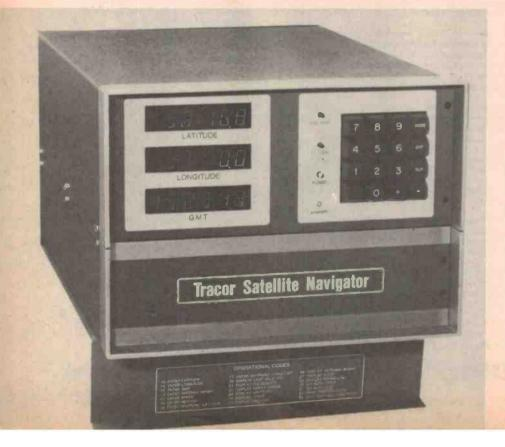
Latitude, longitude and time can be obtained from this satellite navigation system receiver, enabling a navigator to fix his boat's position within a few metres.
