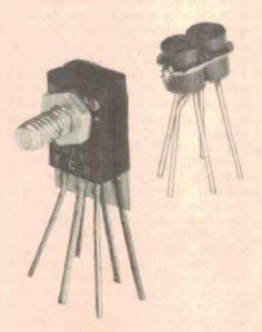
Thermal stabilisation is achieved by mounting the input transistors together as shown and described in the text. Note the insulating piece between the BD140s.
