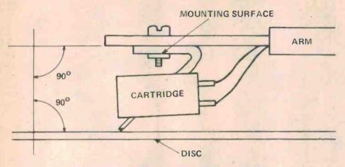
Fig. 2. The cartridge's vertical tracking angle is initially set as shown.
