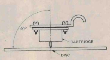
Fig. 1. The stylus must be perfectly vertical in the groove.
