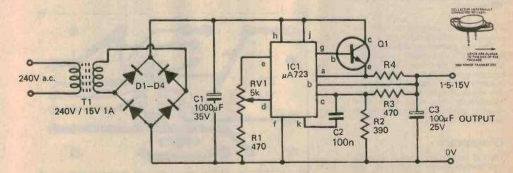
Pin numbers are not shown on the circuit diagram for the regulator IC as either DIL or CAN type packages can be used. A table for pin connections is shown on page 70.
