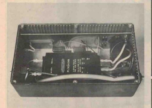
Internal view of the power supply showing how the pc board was mounted, the position of the power transformer and the general wiring arrangement. General parts placement is not at all critical and a variety of layouts is possible. Be sure to insulate the regulator ICs.
