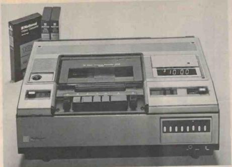
Most of the common video cassette recorders (VCRs) available may be used to record PCM encoded audio when used in conjunction with a special digital processor.
