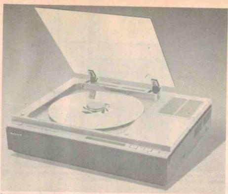
Digital disc systems provide ultra-high density recording — 2½ hours per side for Sony's DAD-1X, and feature claimed dynamic ranges better than 90 dB with THD figures around 0.03 - 0.05%. A helium-neon laser 'reads' the disc in the above machine, signals consisting of 16-bit linear quantized PCM pulses. Surface wear, dust and handling do not affect the discs. Wow and flutter is claimed to be undetectable, even though the disc rotates at 450 RPM!
