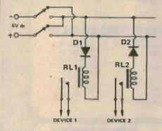
The problem of how to operate two relays independently from just two wires always produces a lot of head scratching — and not just with beginners! This circuit, from the ETI files, shows how it's done.
