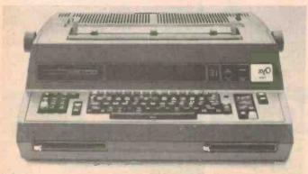
The new Qyx Intelligent Typewriter is available in several different levels, with all levels compatible with the basic unit. Level 1 is a very nice proportional-spacing typewriter with phrase and format recall. centering and self-correction. Level 2 adds a 10 000 character memory and editing features like right margin justification and pagination. Level 3 expands the memory to 60 000 characters and adds some convenience functions, while level four adds a mini-disk drive with 60 K capacity.
